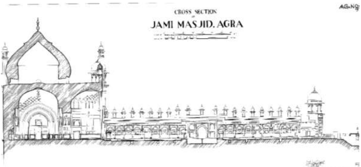
Figure 3 Section through Jama Masjid complex, Source: Archaeological Survey of India, Agra circle, Agra
